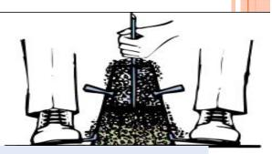
Three layers of approximately equal height in each layer with tin rod 25, but not 25 stokes. Throughout its depth and up to the surface of beneath layer.
