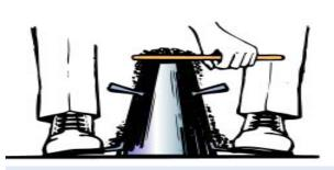
5 Immediately after completion of Ster operation of raising the mold sh performed in 5±2 sec. by a steady upw with no lateral or torsional motion imparted to the concrete. The entire or
