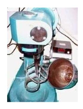
Vicat: Sliding fitting m=300g±1g, testing bar can free fall.
