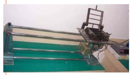
•Vibration compaction sets: Amplitude 15±0.3mm, frequency 60 times /60s±2s.
